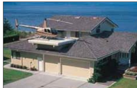
R44 Clipper II, with pop-out floats stowed, on a residential rooftop helipad.
