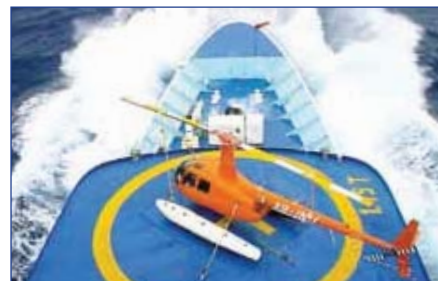
R44 Clipper I shown shipboard with optional rotor blade supports and frame tie-down lugs.
